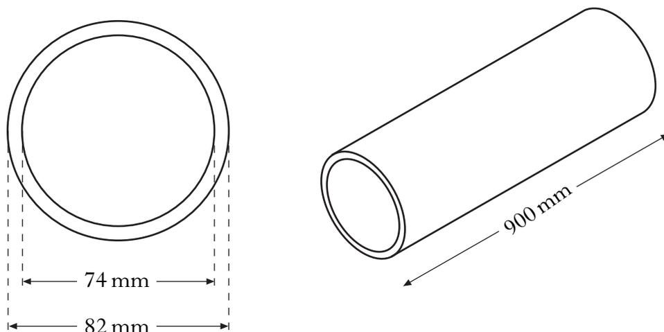
The inner diameter is 74 millimetres.
