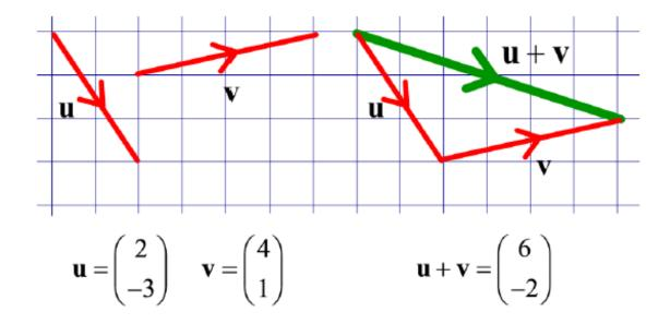
In real life, resultant vectors can be used to work out what the combined effect of more than one force pulling on an object will be.
